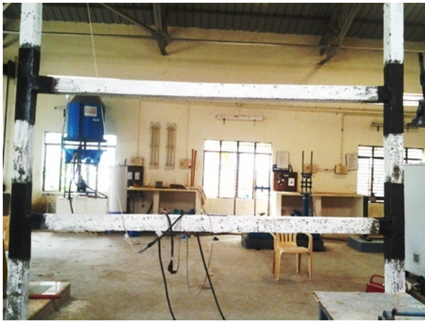
Fig.3(g) Schematic view of retrofitted RC frame
